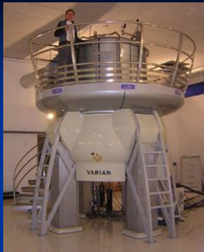
900MHz, 21.2 T NMR Magnet at HWB-NMR, Birmingham, UK being loaded with a sample
