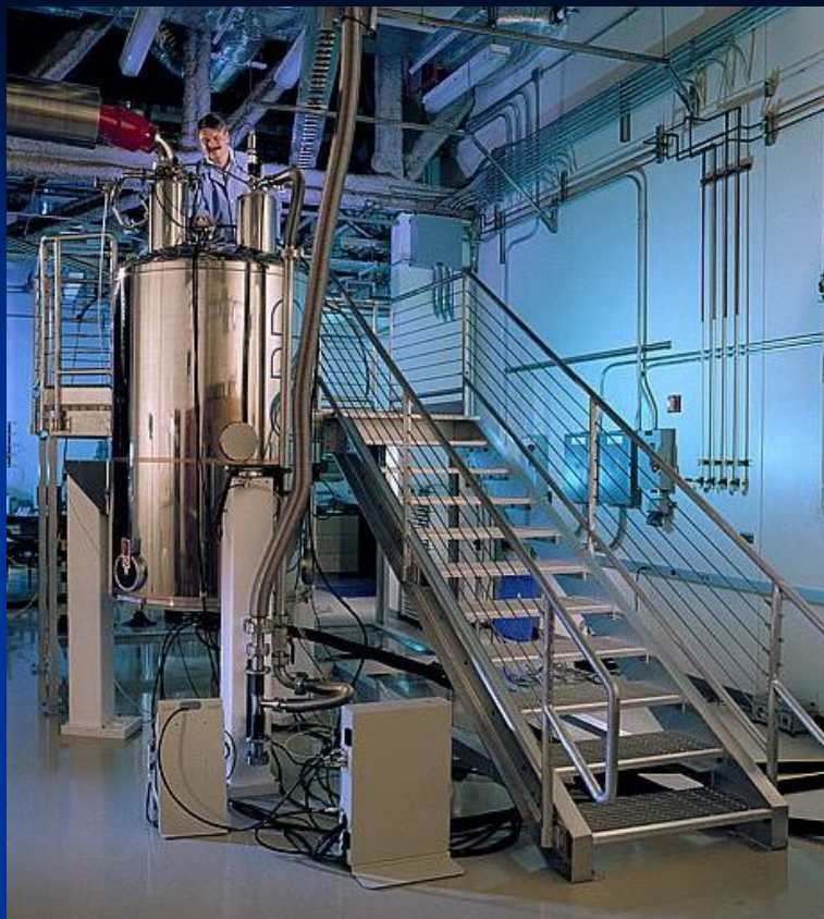
Pacific Northwest National Laboratory's high magnetic field (800 MHz, 18.8 T) NMR spectrometer being loaded with a sample.
